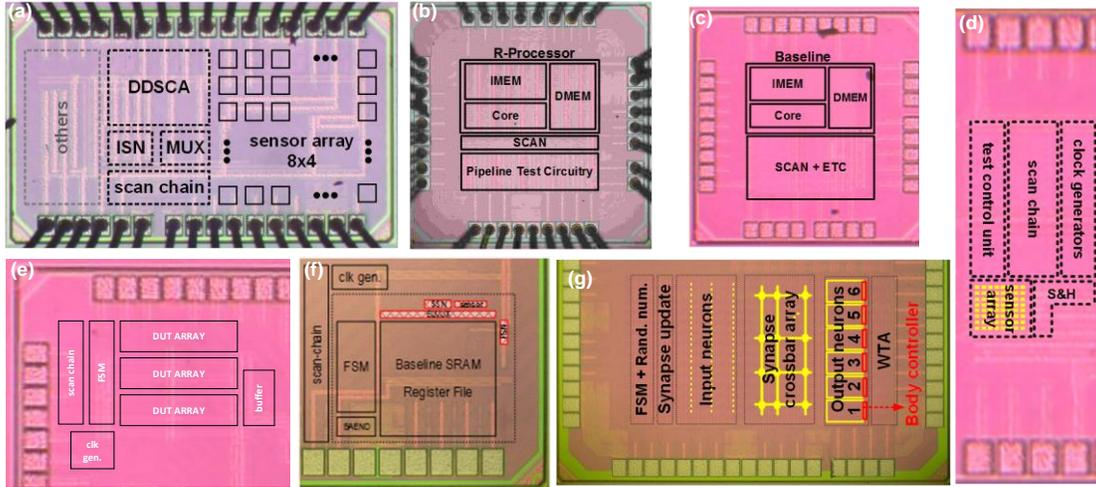
Fig. 1. Die photos of test chips prototyped in this project; (a) [Yang, ISSCC'14 & JSSC'15]; (b,c) [Kim, VLSI'14 & JSSC'15]; (d) [Kim, CICC'15]; (e) [Yang, ISSCC'15]; (f) [Yang, ESSCIRC'16]; (g) [Kim, VLSI'16];
