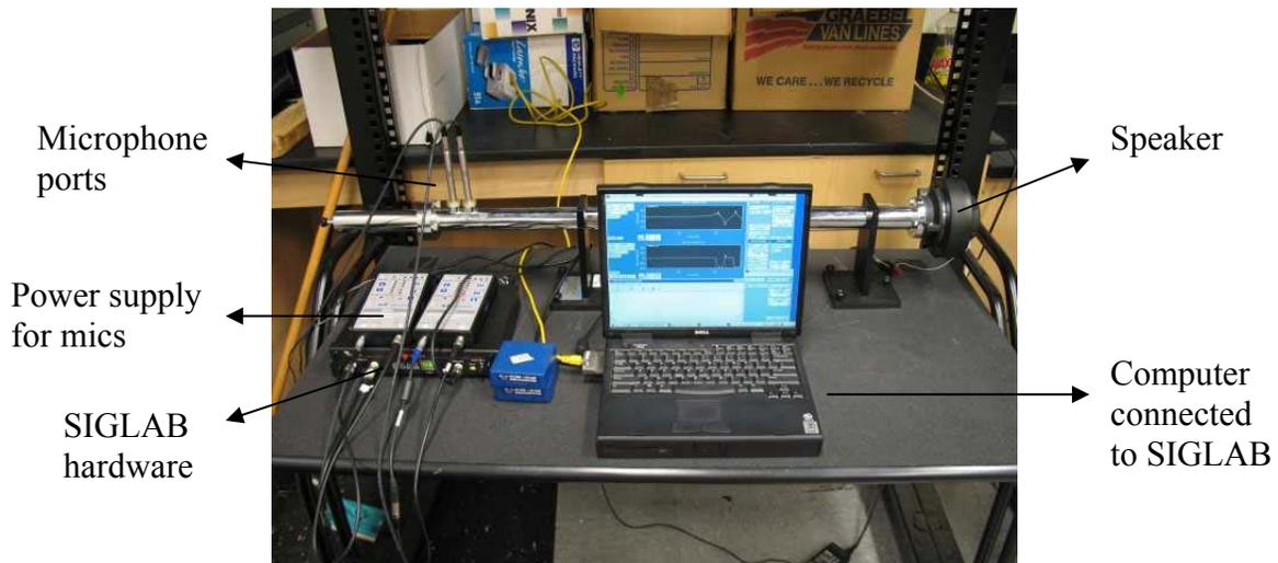
**Figure 2. Picture of the impedance tube experimental setup**
