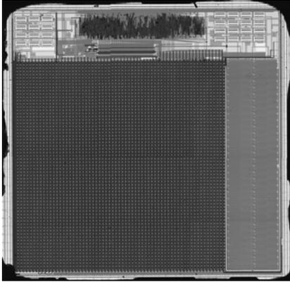
**Figure 4.** Die photo of SPAD array chip.
