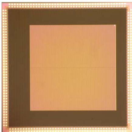
**Figure 1.** Die photograph of active fluorescent microarray chip.
