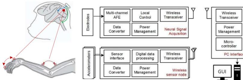
Fig. 1 The SBI system mainly consists of the wearable sensors, neural recorder and neural stimulator.
