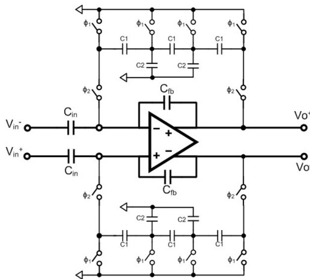
Fig.6. Input amplifier with switched-capacitor ladder
