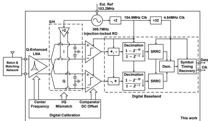
Fig. 4. System block diagram of 2.4GHz sub-sampling DPSK receiver.
