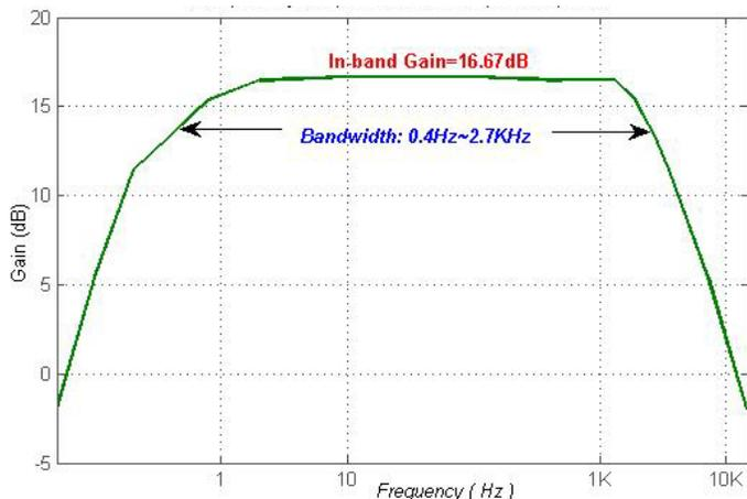
Fig.7. Frequency response of the input amplifier
