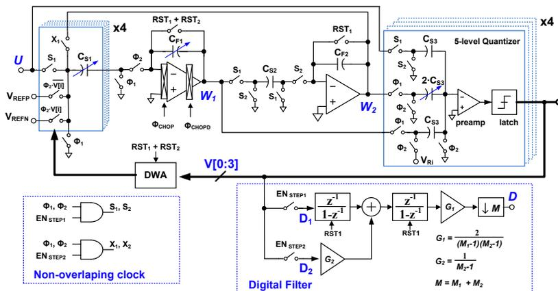
Fig.8. IADC circuit with digital filter.
