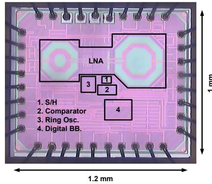
Fig. 5: Die photo of the 2.4GHz sub-sampling receiver.
