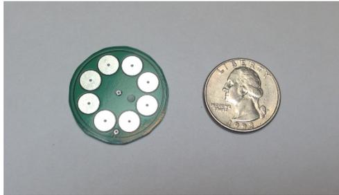
Fig. 2. The bottom side of the sensor showing its circular electrode array
