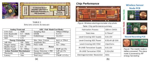
Fig. 2 (a) A wireless bi-directional BMI chip, device and die photo, and table of testing specifications. (b) A wireless body area sensor chip, device and table of testing specifications.
