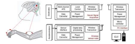
Fig. 1 The SBI system mainly consists of the wearable sensors, neural recorder and neural stimulator.
